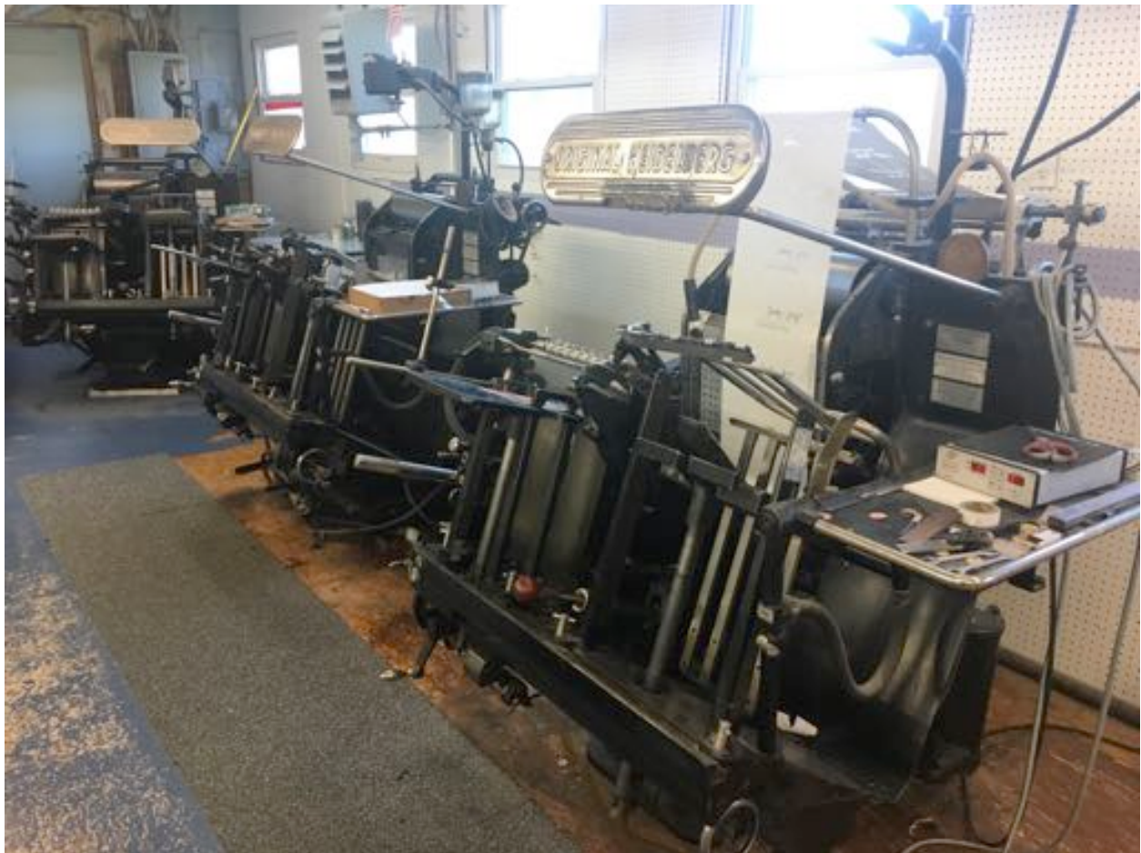
Heidelberg Windmill Presses Prepped for a Hot Foil Job
