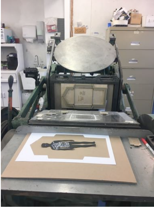
Platen Press from 1920 suited for Die Cut Envelopes
